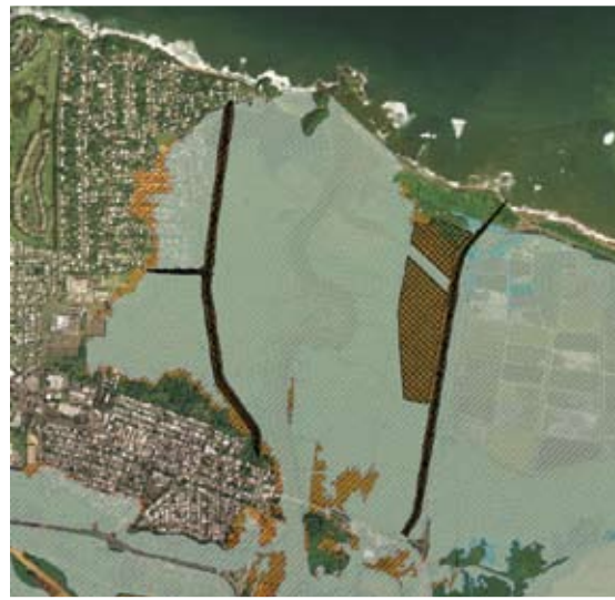
Top: A two-D hydrodynamic model supports a flood risk reduction system for the Rio de la Plata, Puerto Rico.
